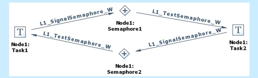
Tasks and semaphore on different nodes Good measure of overhead of kernel + drivers + communication latency
