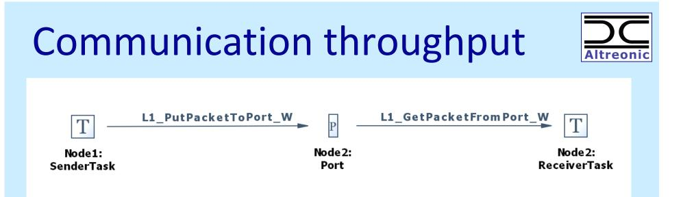
Uses OpenComRTOS packet switching Task synchronise first in Port Hub (=> ACK) Data copied from send packet to receive packet in Port Hub
