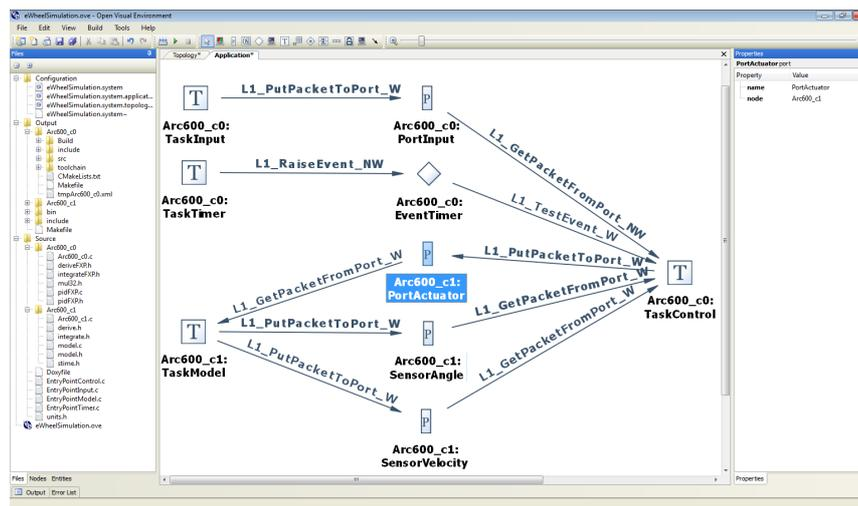
Using metamodeling, embedded software engineers can define their own targets, target topology, application topology. They can graphically create the program code, build and run the executable images. Before the final target is used, they can run the application on a host operating system such as Windows or Linux, allowing them to verify the behaviour. A built in event tracer allows users to verify the scheduling and task interactions. Once done, a small click of the mouse changes the
