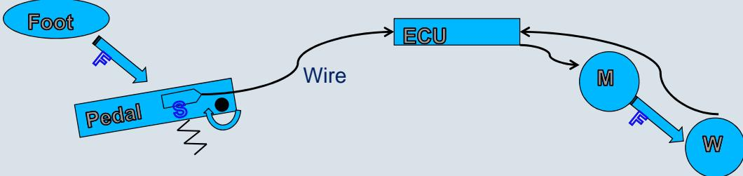
Multiple links between sensor and ECU, each one can fail.
